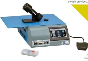
When the animal reaches the threshold of pain and flicks its tail, a sensor detects the tail removal from the heat source and stops the reaction-time counter, simultaneously switching off the bulb.
