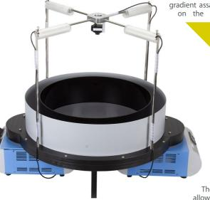
Phenotyping in Mice using an innovative Automated Circular Gradient Assay", published by the University Erlangen-Nuernberg (see Zimmmermann's paper). The new TGR (Thermal Gradient Ring) provides an high degree of freedom, i.e. thermal choice, and eliminates experimenter bias.
