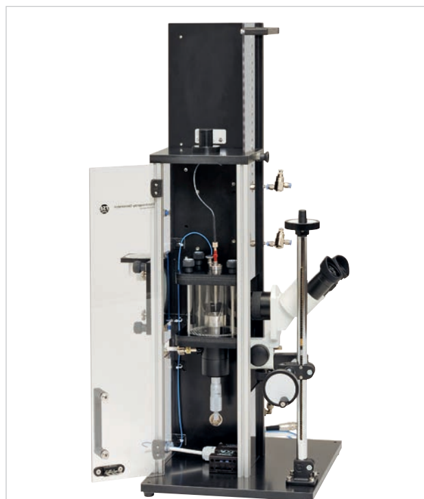
E-Spray NanoGen – in-vitro setup
