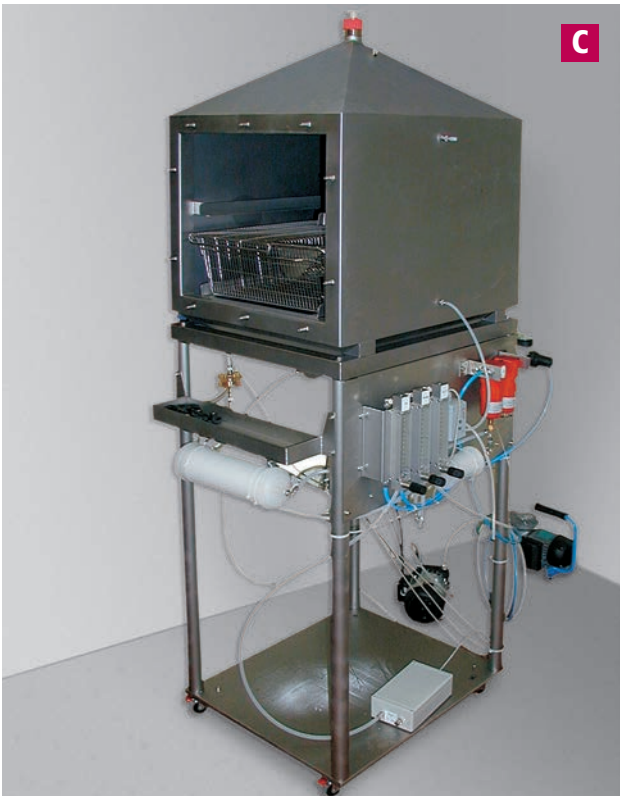
Whole Body Unit for one type 3 cage
