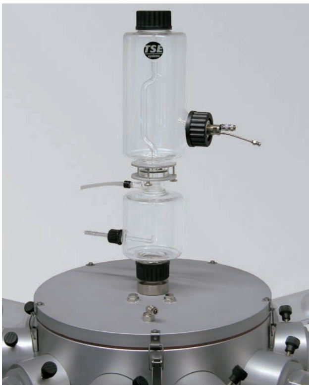
Aerosol nozzle – mounted on preseparator
