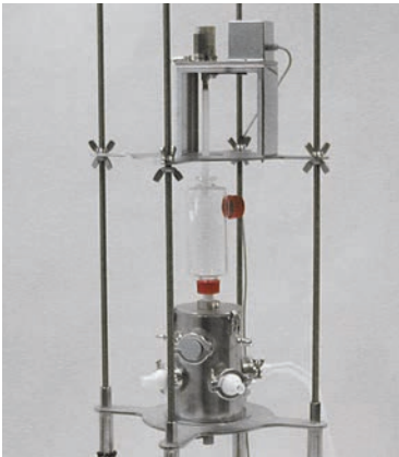
Upper unit with dust generator
