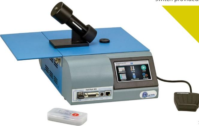
When the animal reaches the threshold of pain and flicks its tail, a sensor detects the tail removal from the heat source and stops the reaction-time counter, simultaneously switching off the bulb. The reaction time of the animal is thus automatically determined to the nearest 0.1 second.
