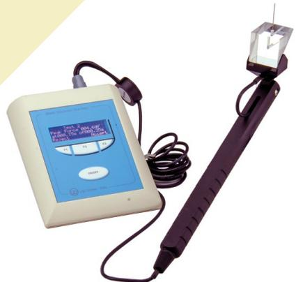
An **Electronic Von Frey** of original design, for automatic assessment of Hypersensitivity and Allodynia in rats and mice, automatically records the animal response to user-controlled application of force rate. A touch stimulator transducer is mounted on a Perspex handle, so that routine procedures may be employed to examine and test the animal skin sensitivity. A proprietary prism is of great help to localize the aimed stimulation area.
