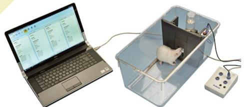
The **Orofacial Stimulation Test** by Ugo Basile is a new method to measure hypersensitivity to thermal or mechanical stimulation of the trigeminal area in rats and mice; animals are trained & tested in standard home cages.
