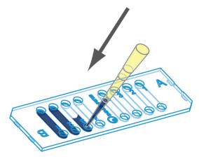
Fill 20 µl into the Smart Slide with a pipet.
