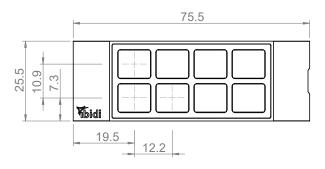
Geometry of the µ-Slide 8 Well <sup>high</sup> Glass Bottom
