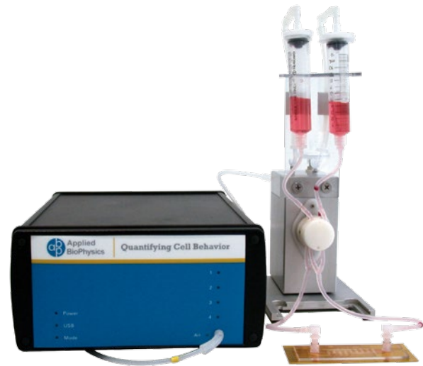
System overview: ECIS Flow Module for the cultivation of cells under flow conditions
