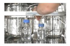
The AVD Series combines all the features of a saturated steam sterilizer with the capability of performing bio-decontamination cycles using VH2O2. Sharing the same chamber, utilities, and control system, this multipurpose device requires less space and operating cost compared with two independent and dedicated unit. Using VH2O2 technology provides a complete turnkey solution for the bio-decontamination of heat-sensitive equipment to be transferred from one classified area to another.
