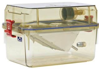
BCU-Mouse cage: This illustrates the description of a biocontainment cage: sealed cage, solid top, locked top, gasketed, exhaust pre filter, sealed intake and exhaust ports.
