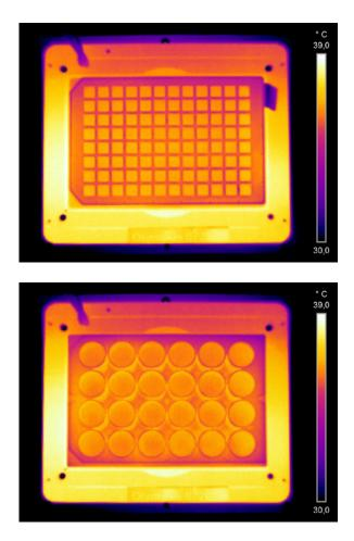
Stable and consistent temperature distribution in every well of multiwell plates in the ibidi Stage Top Incubation System. Images were acquired with a FLIR thermal camera.
